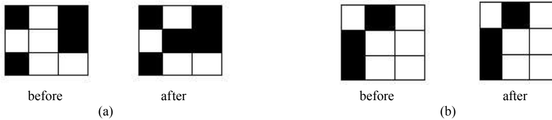
Fig 9: Darkening process (consider middle position) when threshold=3 (a) eligible to be black from white (b) not eligible to be black from white
