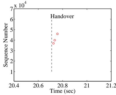
Fig. 6. Retransmissions at CN during M-NEMO handover between homogeneous capacity networks.
