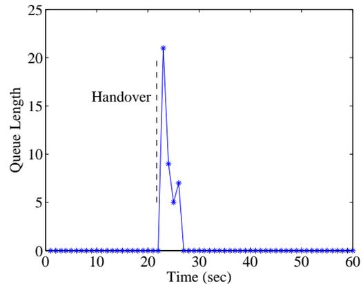
Fig. 18. Queue length at AR<sub>2</sub> for SINEMO handover between heterogeneous capacity networks.
