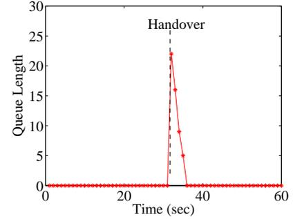
Fig. 7. Queue length at AR<sub>2</sub> during M-NEMO handover between homogeneous capacity networks.
