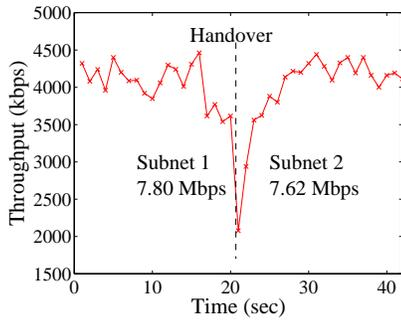
Fig. 5. Throughput at LFN for M-NEMO handover between homogeneous capacity networks.
