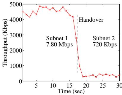
Fig. 11. Throughput at LFN during M-NEMO handover between heterogeneous capacity networks.
