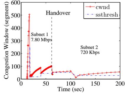
Fig. 13. Congestion window for TCP RENO data source at CN during M-NEMO handover between heterogeneous capacity networks.
