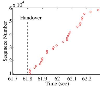
Fig. 12. Retransmissions at CN during M-NEMO handover between heterogeneous capacity networks.
