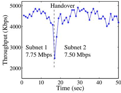
Fig. 8. Throughput at LFN for SINEMO handover between homogeneous capacity networks.
