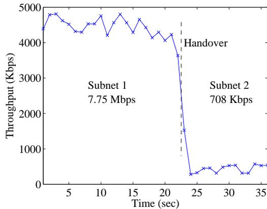
Fig. 15. Throughput at LFN during SINEMO handover between heterogeneous capacity networks.
