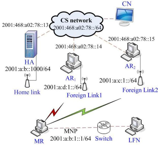
Fig. 3. Experimental testbed for M-NEMO.
