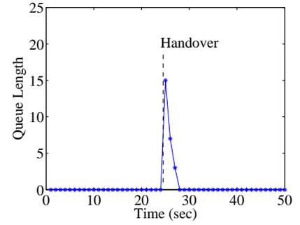
Fig. 10. Queue length at AR<sub>2</sub> during SINEMO handover between homogeneous capacity networks.
