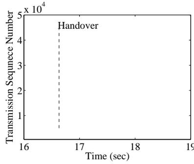
Fig. 9. Retransmissions at CN during SINEMO handover between homogeneous capacity networks.
