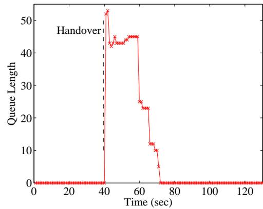
Fig. 14. Queue length at AR<sub>2</sub> during M-NEMO handover between heterogeneous capacity networks.
