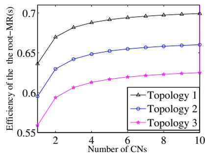
Fig. 8. Efficiency of the root-MR(s) as a function of number of CNs.
