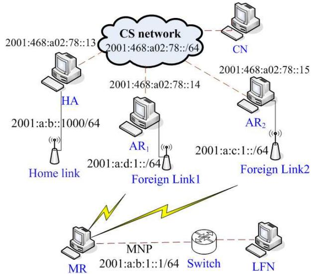
Fig. 4. Testbed Architecture for M-NEMO.
