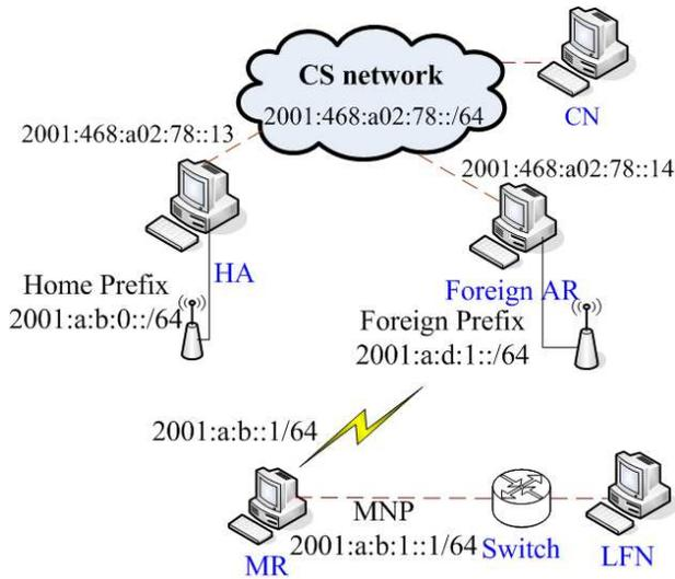
Fig. 3. Testbed Architecture for basic NEMO.
